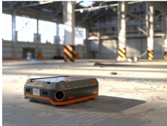
Marking robots can automatically make drawings on the floor.
